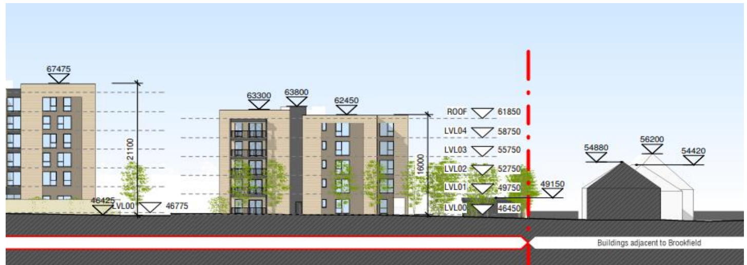
South Elevation Block 4/5 Adjacent to Brookfield
