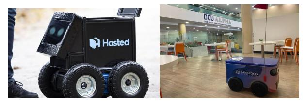
The first robot delivery of a burger and chips to a student was done by the Hosted Kitchens automated Deliver Robot. This relied on teleoperation (driven by a remote driver). While another Delivery Robot from Transpoco (A DCU Alpha company) is piloting AI-enabled Computer Vision to navigate indoors.
