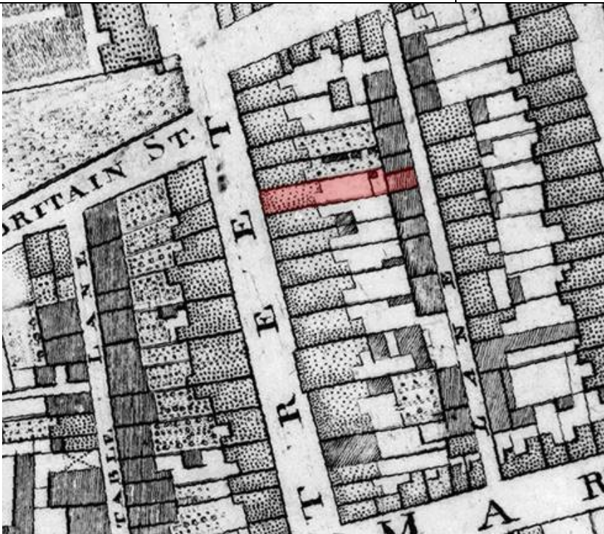
Fig.7: Rocque's Exact Survey of the City and Suburbs of Dublin (1756). No. 56 Capel Street with closet return, rear yard and mews house/outbuilding is hatched red. Note the offset recorded in the rear party boundary between No.56 and No.57 Capel Street, this anomaly remains clearly legible in the current mapping of the site.
