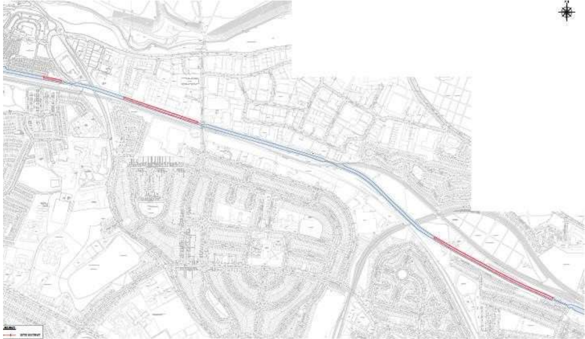
Fig. 2: Sections of Royal Canal Greenway Phase 4 Project for which it proposed to submit an amending Part 8 application (three sections shown in red where it is proposed to narrow the canal/widen the towpath to provide sufficient space for the greenway/cycle scheme).
