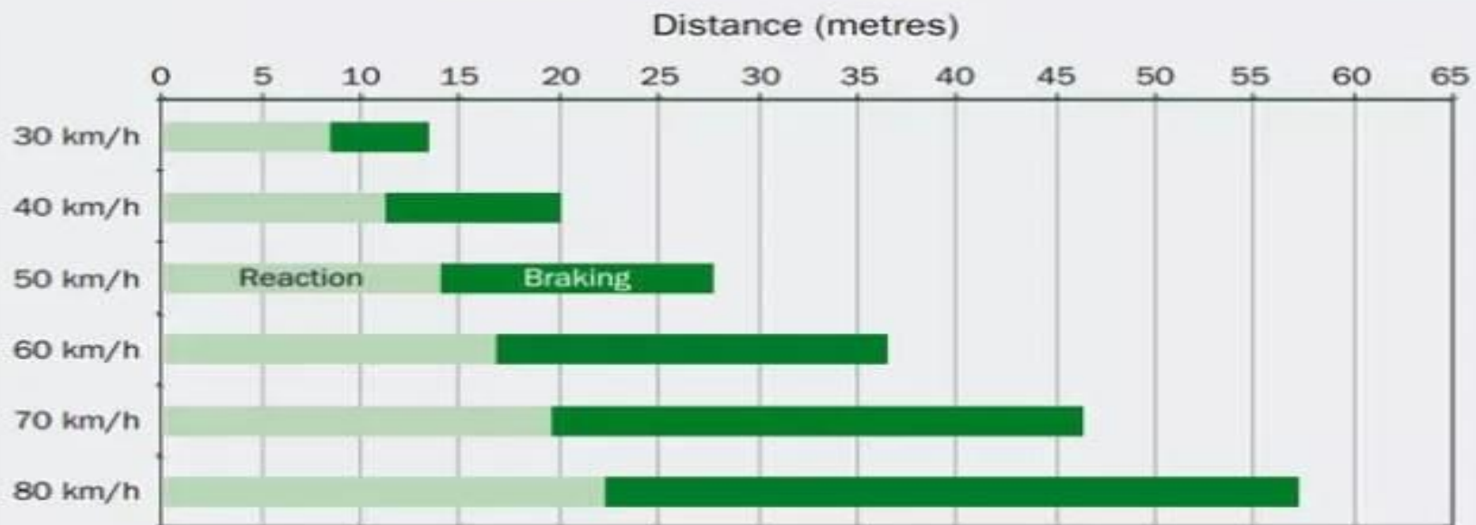
Figure 1.2 Illustration of the stopping distance in an emergency braking
