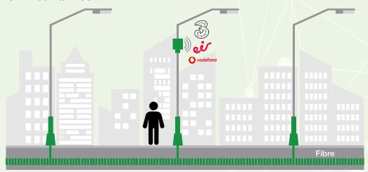
Neutral Host involves a single physical device deployed on city assets that can be shared by multiple operators (as opposed to multiple installations of such equipment).
