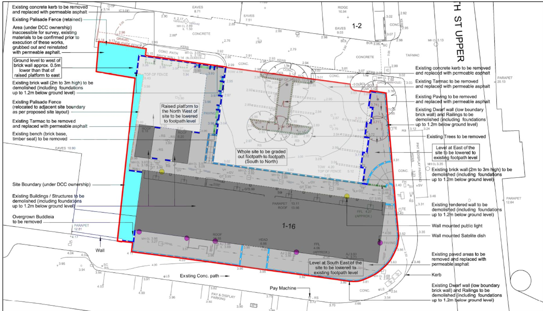
Figure 2. Figure adapted from Drawing SAC-DCCA-XX-XX-DR-CS-1002 (Rev P01) detailing the proposed works at St. Andrew's Court.
