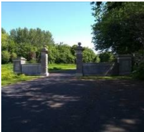
View of southwest side of Neoclassical Northern Gateway, with curving ashlar wall with tall elegant gate-pier and curving ashlar wall terminated by a squat, wide pier. Gate piers display vermiculated rustication.
